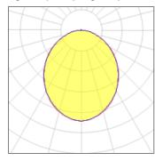
Lamp type Nominal lamp power Total flux Luminous efficacy LED 47 W 4400 lm 94 lm/W CCT
