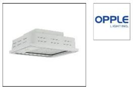
Housing: PC Mounting ring: white; Installation: recessed mounted Dimensions: 421\*400\*95mm Ceiling cutouts: 360\*360mm Power: 120W; Efficacy: 100 Lm/w Lamp(s): Colour temperature: 3000K; Colour rendering: RA80; Total luminous flux of luminaire: 12000Lm Beam angle: 100° Glare control: UGR/; Service life: 60000 Degree of protection: IP65; Class of protection Mains voltage: 220-240V/50-60Hz; surface mounted
