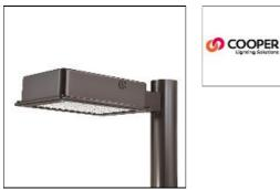
One-piece, die-cast aluminum housing can be pole or wall-mounted, Optical design creates consistent distribution and scalability, Choice of 12 high-efficiency, patented AccuLED Optics<sup>™</sup>, Standard in 4000K (+/- 275K) CCT and nominal 70 CRI, Suitable for operation in -40°C to 40°C ambient environments, 120-277V 50/60Hz, 347V 60Hz or 480V 60Hz operation, Proprietary circuit module withstands 10kV of transient line
