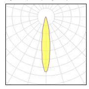
LED CCT 0 K Lamp type Nominal lamp power 63 W CRI -29 Total flux 1660 lm LOR 100% 26 lm/W 63 W Luminous efficacy Total power
