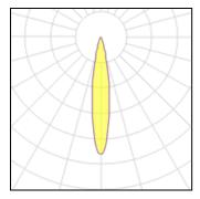
Lamp type LED CCT 0 K Nominal lamp power 82 W CRI -50 Total flux 630 lm LOR 100% Luminous efficacy 8 lm/W Total power 82 W
