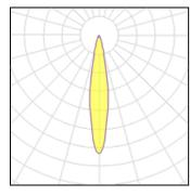
CCT 7247 K Lamp type LED Nominal lamp power 85 W CRI -18 3220 lm Total flux LOR 100% Luminous efficacy 38 lm/W Total power 85 W
