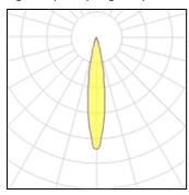
CCT Lamp type LED 6500 K Nominal lamp power 80.5 W CRI 70 Total flux 4510 lm LOR 100% Luminous efficacy 56 lm/W Total power 80.5 W
