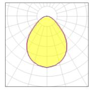
Lamp type Nominal lamp power Total flux Luminous efficacy LED 47 W 4000 lm 85 lm/W CCT
