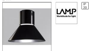
Suspended downlight model STORMBELL 5000 WW WFL BK/WH., LAMP brand. Made of shiny black extruded and injected aluminum body with polycarbonate opal ring. Model for COB with warm white color temperature and control gear included on white decorative rose. Wide Flood aluminum reflector. Insulation class I.
