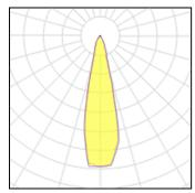
1 x LED Nominal lamp power 52 W LOR 71% Lamp flux 8550 lm Total flux 6070 lm Luminous efficacy 164 lm/W Total power 56 W CCT 3000 K CRI 80
